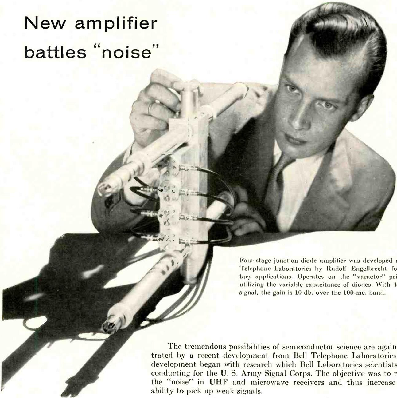
Four-stage junction diode amplifier was developed at Bell Telephone Laboratories by Rudolf Engelbrecht for military applications. Operates on the "varactor" principle, utilizing the variable capacitance of diodes. With 400-mc. signal, the gain is 10 db. over the 100-mc. band.
