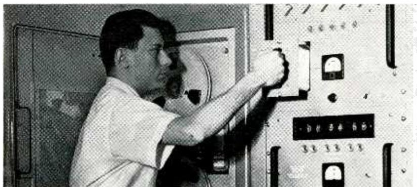
Engineer inserts 60- and 30-ips speed playback hand-pass filter into magnetic tape search unit. Digital timing generator is below search unit
