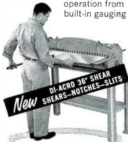
New cam-lever linkage of the Di-Acro Model 36 shear provides a greater mechanical advantage than lever actions. This makes it easier to control both machine and material so that operation is easier, faster and safer.
