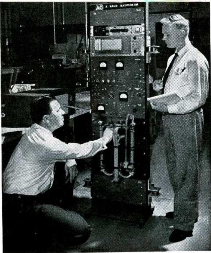
Authors are calibrating the radiometer with dummy antenna at  $-18\text{ C}$
