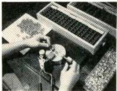
Jig bends leads of diodes into position
