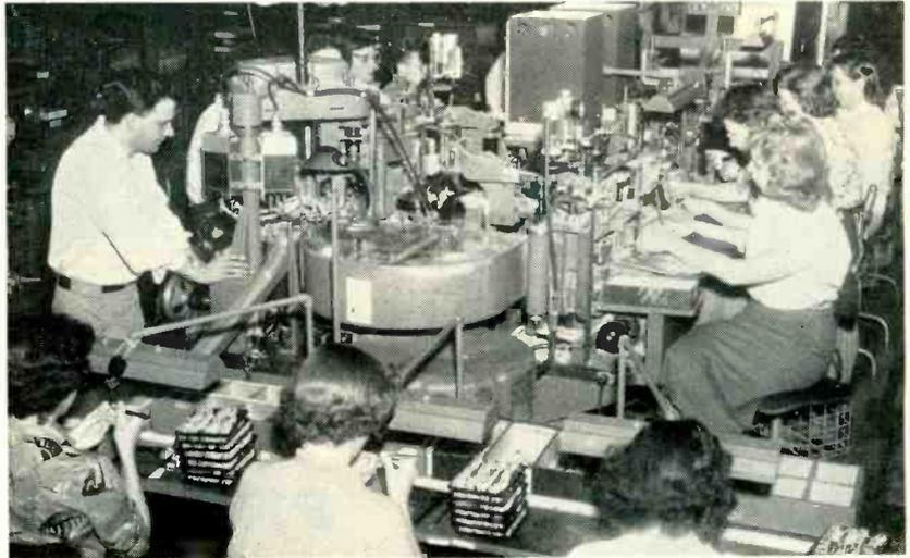
At top speed, this tube cage assembly machine represents a production rate of more than 100 assemblies an hour for each operator required
