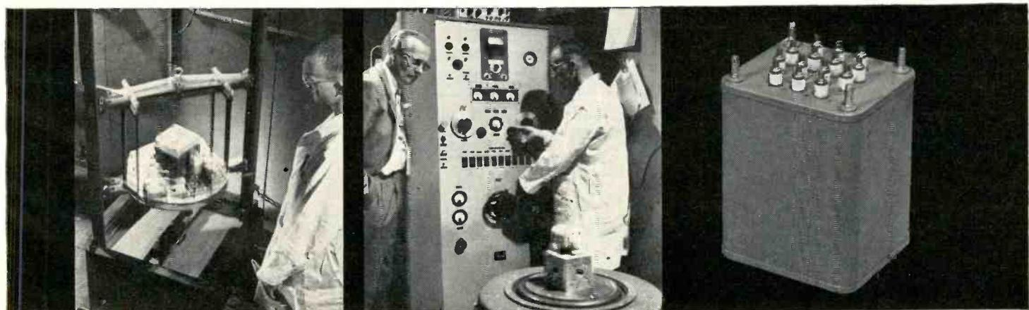
Westinghouse electronic transformers being shock-tested according to specifications of MIL-T-27A with new in-plant qualification testing equipment.
