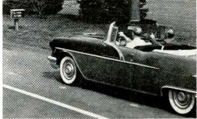
Illuminated sign actuated by RCA's roadside signaling system advises driver his car is exceeding speed limit
