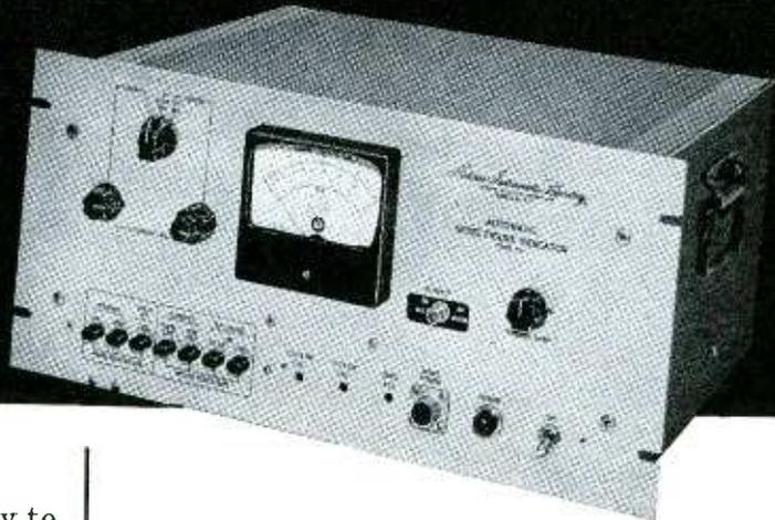
Adding new versatility to your Automatic Noise Figure Measurement equipment, AIL now offers the outstanding Type 74 Automatic Noise Figure Indicator with a tunable Frequency IF Amplifier...or you can purchase the Tunable IF Amplifier for modification of your present Type 74 equipment.
